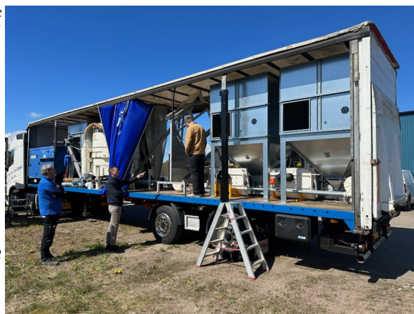
Figur 3: The first inspection of the sensatinoal new equipment of a mobile factory with single seed sorting with NIT analysis with a capacity of 4 tonnes per hour
